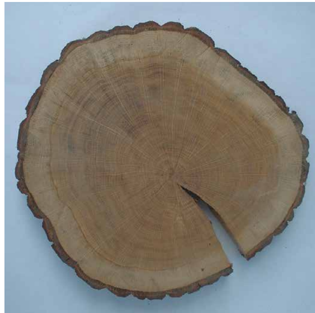
Figure 4: Tangential shrinkage causes a fissure between the heart of this sample and its bark
