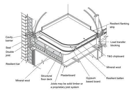
Figure 7: Party floor with solid timber joists
