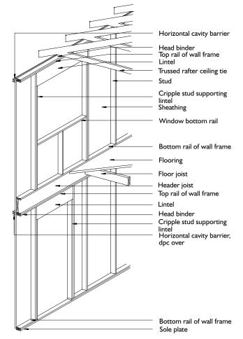
Figure 4: Typical external wall construction
