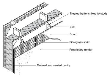
Figure 6: External wall with proprietary render system on backing board
