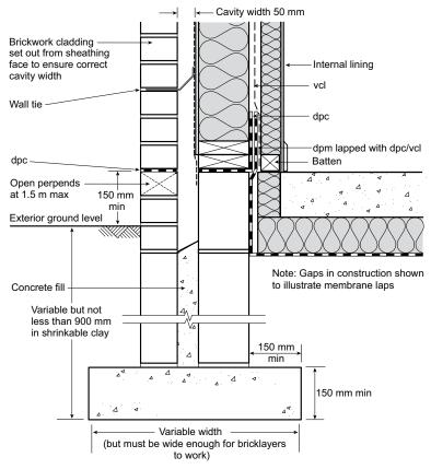
Figure 8: Strip foundation with masonry cladding
